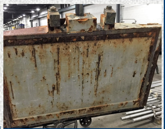
A 40-yr old gate disc before refurbishing.
