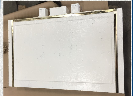
Gate disc (above) and frame (below) after being sandblasted, coated, seats weld-repaired and machined to meet AWWA leakage specs.
