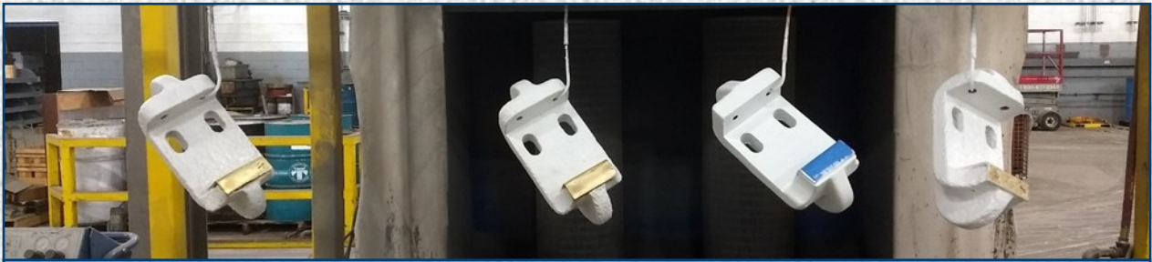
Gate top wedges (three refurbished and one new) after coating.
