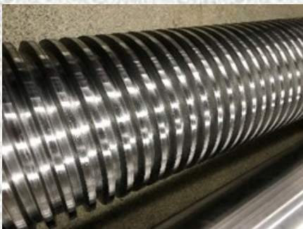
A 10"-1 TPI stem with a 16 Ra finish.
